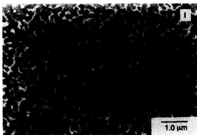
Figure 9 TEM micrographs of epoxy/DDS/PES/PES-OH = 47/23/10/20; epoxy and PES-OH pre-reacted at 180 °C for 3 h and then cured with DDS at 180 °C for 3 h (resin I)
